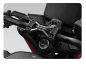
HANDLE HOLDER 08F71-MLB-D00 Precision-cut aluminium handlebar holder featuring the Hornet logo that provides additional high-quality appearance to the CB750 Hornet.
